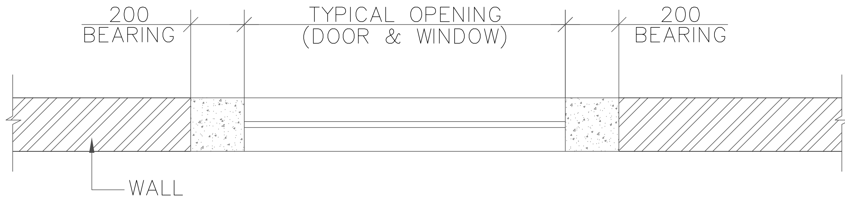
TYPICAL CHEJJA PLAN AT LINTEL LEVEL
